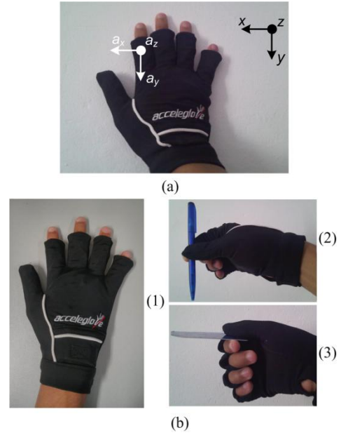
Fig. 2. Master unit. (a) Reference system and kinematic variables of Acceleglove. (b) Therapist hand in the three admissible configurations. (1) "Rest". (2) "Pinch". (3) "Lateral grasp".
